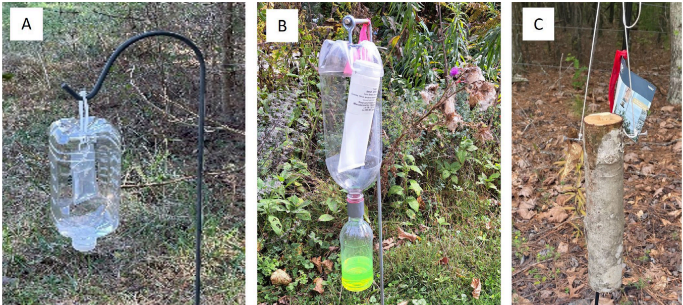
FIGURE 1 | (A) Non-tornado square bottle trap with low release ethanol lure. (B) Tornado round bottle trap with high release ethanol lure, and (C) cored bolt. Photo credits (A) Shimat Joseph (University of Georgia), (B) Aaron Yilmaz (USDA-ARS), and (C) Zia Williamson (University of Georgia). [Colour figure can be viewed at wileyonlinelibrary.com ]
